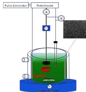
Ni/graphene coatings are produced using a Watt's type bath by applying both direct and pulsed current conditions, in presence or absence of additive in the electrolytic bath. The imposed current pulses ranging between 0.1 up to 1000 Hz, while the duty cycle is kept constant and equal to 50%. The surface morphology, the crystallographic orientations, as well as the mechanical properties are investigated.
