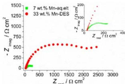
**Zn-Mn coatings are electrodeposited from choline chloride-urea deep eutectic solvent (DES).** Well adhered, homogenous coatings are obtained at current densities up to 8 mA cm<sup>-2</sup>. The corrosion stability of these deposits is compared with coatings deposited from a conventional water-based electrolyte. Deposition from DES enables incorporation of greater Mn amounts which, in turn affords superior corrosion resistance.
