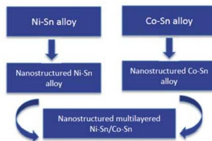
**Starting from 3 metallic elements, namely Co, Ni, and Sn, different types of coatings with different compositions and/or structures can be electroplated.** Such types are single elements, binary alloys, intermetallic, multilayered or gradient coatings. An overview will be given. Design tools are not yet available for selecting most promising combination of these three elements, and that problem will become even more complex for ternary alloys.
