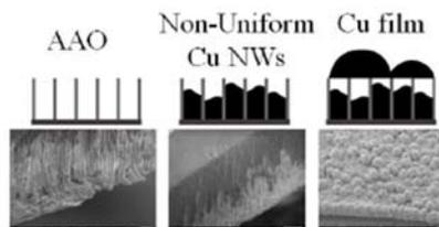
**Copper nanowires were fabricated by filling commercial AAO nanochannels by utilizing Direct and Pulse Current Electrodeposition.**
