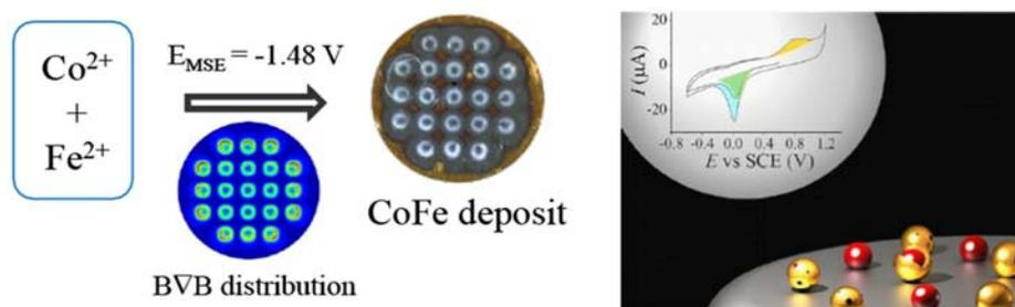
Fig. 1: Magnetic field controlled structuring of electrodeposits (left) and electrochemical characterization of magnetic core shell nanoparticles (right)
