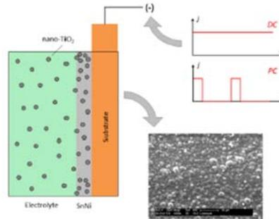
**Tin-nickel alloy coatings with dispersed nano-scaled TiO<sub>2</sub>-particles are fabricated by electrodeposition using DC and PC plating.** Properties and composition of the layers are examined. The average titanium dioxide content is 1.4 wt-%, while the ratio of tin and nickel remains almost constant. Besides the equimolar phase NiSn, other tin-nickel phases are observed in both pristine tin-nickel and dispersion coatings.
