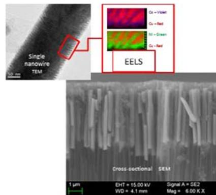
**Ni-Co/Cu multilayered nanowires were fabricated by template-assisted nanowire growth from an optimized aqueous electrolyte by using two-pulse plating.** The magnetic (Ni-Co alloy) / non-magnetic (Cu) nanowire segmented structure was achieved during growth along the length of the nanowires. Structural characterization of the nanowires was carried out using SEM, TEM and EELS techniques. (Work is outcome of an STSM.)
