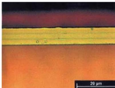
**Pd and Fe were electrodeposited from a stable aqueous electrolyte.** Tear-free layers show a laminar structure with small grains and good corrosion resistance. Complete solid solution of Pd and Fe is deposited as a fcc and bcc crystal structure depending on the composition. Deposits show promising properties in a wide range of composition including expected excellent magnetic properties.
