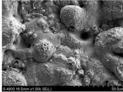
**Surface modification of inert particles allows the structural modification of plasma electrolytically formed layers.** While classical PEO coatings will provide excellent surface hardness and resistance against abrasion, the corrosion resistance is low due to pores and other structural defects. This problem can be overcome by the incorporation of particles in combination with high frequency pulses.
