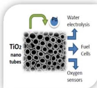
**Pd nanoparticles are deposited onto WC based and 3D - TiO<sub>2</sub> oxide nanotubes supports, to obtain high surface area catalysts for electrochemical conversion systems.** The synthesized materials are characterized by XRD, HRTEM, EELS, XPS and electrochemical techniques. Pd particles size of a few nm is estimated, even the clusters of Pd atoms. The catalytic activity for the oxygen reduction and hydrogen evolution are studied.
