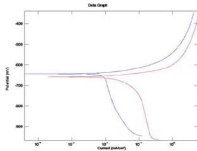
**Aluminium-graphene composites were prepared over a range of compositions.** These were then subjected to potentiodynamic polarisation in neutral aerated 0.1 mol dm<sup>-3</sup> NaCl electrolyte. The corrosion characteristics of the composites were inferior to pure aluminium, possibly due to the influence of the graphene on both promotion of the oxygen reduction reaction and/or a microgalvanic effect.
