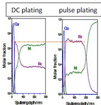
**The reverse composition depth profile of electrodeposited Ni-Fe films was investigated by secondary neutral mass spectroscopy (SNMS).** For DC plating, a strong composition profile was found which extended up to about 100 nm depth. With appropriate pulse-plating conditions, the composition profile remained homogeneous over the entire thickness. This helps achieving better soft magnetic properties (lower coercive force).
