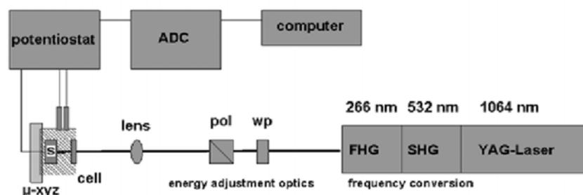
Fig. 1: Electrochemical ns-UV-laser-depassivation setup (266 nm). s: sample. Pol: polarizer. wp: waveplate.)
